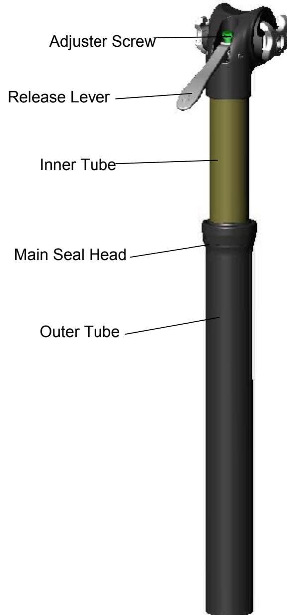
**NOTE:** In some rare cases, your seatpost may “bounce” back up when placed in the lowest position. This is normal and is caused by a pocket of air that is pressurized when the seatpost is lowered. To fix this, simply loosen the Main Seal Head and lower the seatpost. With the seatpost in the lowered position, hand tighten the Main Seal Head.
