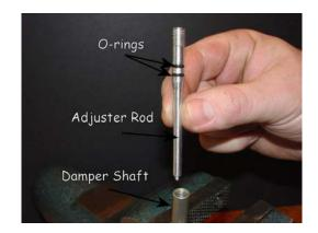
4.4.8. To remove the Internal Floating Piston (IFP), clamp the Damper Tube in a vice with 22mm Shaft Clamp Blocks and unthread the Attachment Boss using a 21mm wrench. The IFP can be pushed out the bottom.
