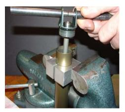
4.4.4. Loosen the Seal Head by clamping the ML7.2 damper tube in a vise using the Maverick 22mm vise clamps, 25mm below the top edge of the damper tube. Unscrew the Seal Head from the Damper Tube. Drain the Oil and discard of properly.
