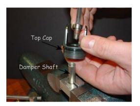
4.4.7. If needed, the Adjuster Rod can be removed from the Damper Shaft by threading it out with a 3mm Hex key. When replacing, grease the O-rings and make sure they are not damaged when passing through the threaded portion of the Damper Shaft.
