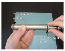
5.2.4. Install the attachment boss and tighten both it and the seal head to 6NM.
