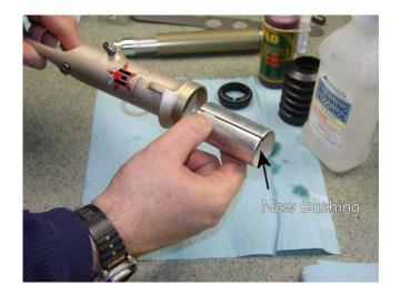
4.3.6. Once in place, the Bushing will need to be sized with the Maverick Bushing Tool. This is done by pushing the bulged end of the tool through the bushing several times. Lubricate the Bushing beforehand with grease or Gunna-Flow.
