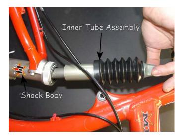
4.1.6. To re-install, position the bike so the Shock Body is horizontal. If the Lubrication Oil has been cleaned out, add 6ml of Maverick Gunna-Flow lube into the Shock Body. Smear another 1ml of lube to the Wiper, Main Seal and Bushing.
