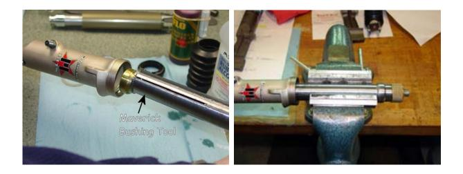
If the bushing is too tight to remove while the Shock Body is in the frame, remove it and clamp the Bushing Tool into a vice. Use a vice with soft "V" shaped jaws. *Be careful not to damage the bulged end of the tool in the vice*.
