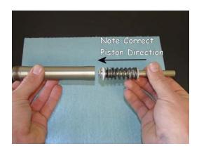
5.2. To assemble the Cartridge, first install the Piston/Damper Shaft/Seal head assembly into the damper tube with no oil and the IFP and attachment boss removed. Thread the Seal head in only up to where the O-ring touches the Damper tube. It will be tightened later.
