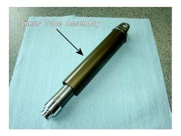
4.4.2. Using a 4mm hex key, loosen (do not remove) the Set Screw located at the center of the Attachment Boss on the bottom of the Cartridge. This will allow the air pressure charge to be released. CAUTION: Contents under Pressure!!!! BE SURE the air is released before Continuing.
