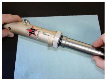
NOTE: Before assembly, inspect inner tube for any knick, scratches, or imperfections on the surface that would prevent a perfect Seal.
