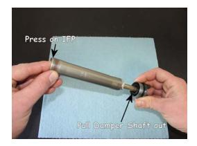
5.2.3. The correct position of the IFP must now be set. With the shaft at Full Extension back out the seal head (not all the way) and pressing the IFP into the cartridge. Oil should escape out around the seal head threads as you are doing this. NOTE: The IFP should be set at 6-8mm from the end of the damper tube when the damper shaft is all the way out and the seal head is tightened against the damper tube.
