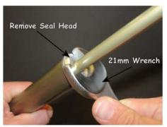
Remove the Seal Head with a 21mm wrench. It may be necessary to clamp the shipping axle into the Drop Out.
