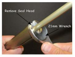
Unscrew the Seal Head using a 21mm wrench. It may be necessary to hold the Damper Tube in a vise (or with a wrench) across the flats.
