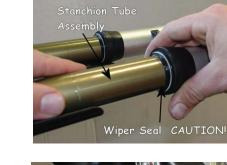
REINSTALL THE DAMPER CARTRIDGE - Insert the Stanchion/Damper Cartridge assembly into Upper tube.
