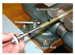
Be careful of the O-rings on the Lock Tube. Insert the Rod slowly and press O-rings down with small Allen wrench to prevent their catching on the holes in the Damper Shaft.
