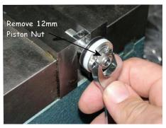
To disassemble the Piston and Shims, clamp the Piston Stud in a flat jawed vise and loosen the Piston Nut.
