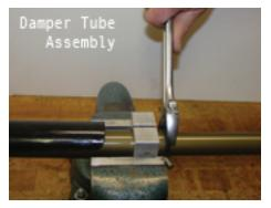
Gently clamp the Damper Tube in a 32mm vise clamp wrench and unscrew the Stanchion Tube.
