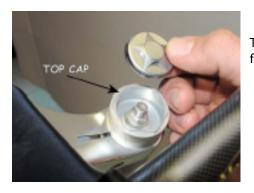
The fork Top Cap should not be removed for regular service.
