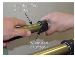
Insert the Stanchion assembly into the Upper Tube. A small amount of lubrication oil should be first wiped on the seals.
