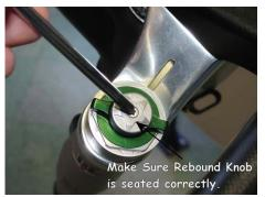
When connecting the Rebound Knob, be sure it connects properly with the flats on the Adjuster Rod.
