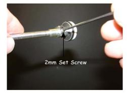
With a 2mm hex key, unscrew the Lock Tube Pin from the Piston Stud.
