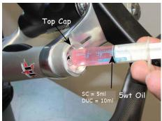
Before pushing the Damper Rod all the way into the Top Cap, inject 5 wt lube oil through the bolt hole for bushing lubrication. SC = 5ml; DUC = 10ml
