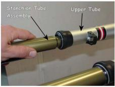
Pull the Stanchion Tube and Air Spring Assembly out of the Upper Tube.
