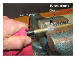
If it is necessary to remove the Air Piston, hold the Rod with a 10mm shaft clamp (available from Maverick) and turn the Piston by holding it with a rag. The threads are Locktited, so it will be hard to turn.
