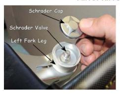
Remove the Schrader Cap on the left side of the fork and release the air pressure.
