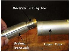
Pull the bushing out of the Upper Tube.
