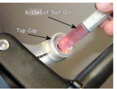
Before pushing the Air Spring Rod all the way into the Top Cap, inject 8-10 ml of 5-7 wt lubrication oil through the bolt hole. Do not inject the oil into the Air Spring Rod
