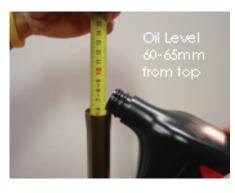
Once the parts are reassembled, fill the empty Damper Tube with 5wt oil. The amount of oil is determined by the level it is from the top of the empty Damper Tube. The correct level is 63 mm from the top of both the DUC & SC.
