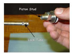
The Lock Tube can now be separated from the Piston Stud.
