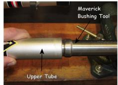
Check the fit of the Stanchion Tube inside the installed Bushing. If it is tight, the Bushing will need to be "sized".
