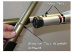
Pull the Stanchion Tube Assembly out of the Upper Tube.
