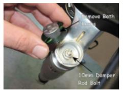
Remove the Damper Rod Bolt using a 10 mm socket.
