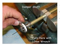
Adjuster Rod and Lock Tube Removal:
