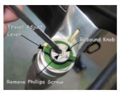
Remove the Phillips screw to take off the two knobs.
