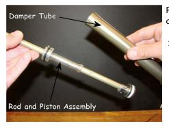
Pull the Rod and Piston and Rod assembly out of the Damper Tube.
