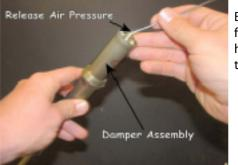
Before disassembling the Damper, first release the air pressure inside by holding the cartridge upside down and then depressing the Schrader valve.
