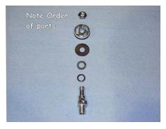
Be sure to note the direction of the Piston and order of the Shims when disassembling.
