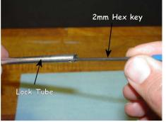
The Adjuster Rod has a 2mm hex socket at the bottom end for removing it from the Lock Tube. Insert a hex key into the bottom end of the Lock Tube and engage it with the Adjuster Rod.
