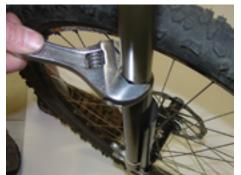
An alternate way to separate the Damper and Stanchion Tubes is to clamp the Stanchion to the axle.
