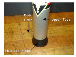
To install a new Seal Head, spread a small amount of blue Locktite\* on the outer surface of the Upper Tube and push the Seal Head on as shown.
