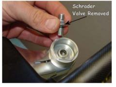
Remove the Schrader Valve with a 10mm socket.
