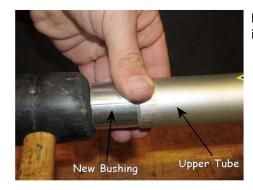
Install the Bushing by gently pushing it into the Upper tube.
