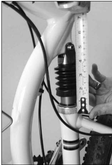
Approximate Pressure Settings for Rider Weight (Use sag measurements for best performance)
